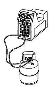
To start you must have a minimum of 5 lbs. of liquid refrigerant in the tank.
